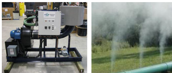
All Natural: The odor reduction system implemented at the mill disperses a non-toxic vapor that absorbs and removes odors.
